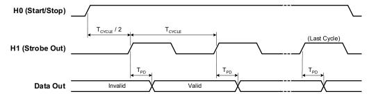
Optionally, you can provide an *external* strobe input on the H2 line to control the memory transfers. If you pace the memory inputs from an external clock, the 34950A will sense the leading edge of the strobe and set the data. The data will be valid after  $T_{PD}$  and the receiving device may latch the data.  $T_{PD}$  ranges from 82 ns to 47 ns.
