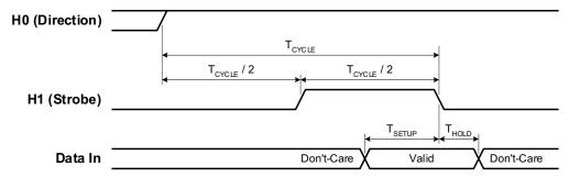
For example, the following SCPI commands set a 34950A in slot 5 to have a 16-bit input using synchronous handshake. Two data inputs are then performed and the strobe line is pulsed for each query. The I/O direction line is set high following the first SENSe:DIGital:DATA:WORD? query and remains high until the digital channel is reset or reconfigured.
