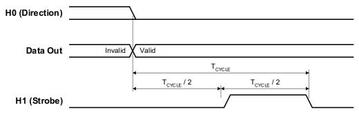
For example, the following SCPI commands set a 34950A in slot 5 to have a 16-bit output using synchronous handshake. Two data outputs are then performed and the strobe line is pulsed for each. The I/O direction line is set low following the first SOURce:DIGital:DATA:WORD command and remains low until the digital channel is reset of reconfigured.
