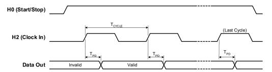
For example, using the *internal* strobe, the following SCPI commands set a 34950A in slot 5 to have a 32-bit output using synchronous handshake. The number of times to output the traces is set to 4. A trace is then loaded into memory and assigned to the channel. The memory is enabled and then triggered. The start/stop line is set high following the first byte handshake and remains high until the last byte is output.
