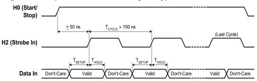
For example, the following SCPI commands set a 34950A in slot 5 to have an 8-bit input using synchronous handshake with an external strobe input. The number of bytes to read into memory is set to infinite (continuous reading into memory until the memory is stopped). The memory is enabled and then triggered. The start/stop line is set high following the first byte handshake and remains high until the last byte is captured.
