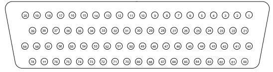
P1 (Bank 1) Connector Pin Assignments
